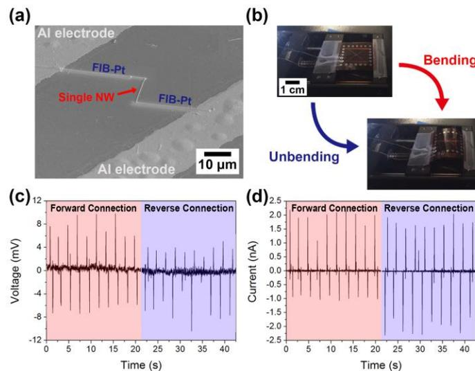
**Figure 3.** (a) SEM image of BaTiO<sub>3</sub> single NW transferred onto an Al patterned flexible substrate by FIB-Pt deposition process. (b) The captured photographs of a single NW-based flexible PEH after and before being deformed by a bending machine. The output voltage (c) and current pulse (d) generated from a BaTiO<sub>3</sub> single NW during mechanical bending/unbending motions in forward and reverse connections, respectively.
