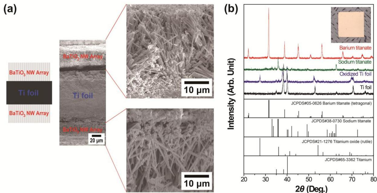
**Figure 2.** (a) The cross-sectional SEM images of BaTiO<sub>3</sub> NW arrays grown onto top and bottom surfaces of a Ti substrate. (b) XRD patterns of the resultants obtained from at each step.
