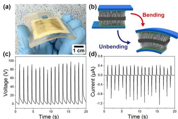
**Figure 4.** (a) Photograph of BaTiO<sub>3</sub> NW arrays-based PEH (3 cm × 3 cm) bent by human fingers. (b) Schematic of NW arrays-based PEH under original (releasing) and bending states. The output voltage (c) and current (d) converted from mechanical deformations by human fingers.
