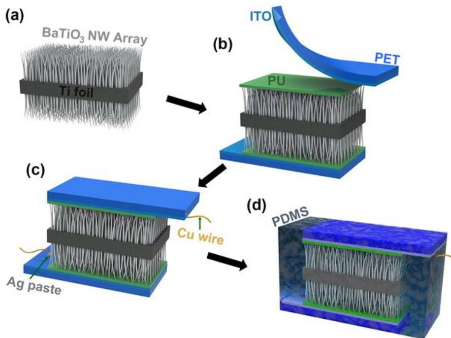
**Figure 1.** Schematic illustration of overall fabrication process of vertically grown BaTiO<sub>3</sub> NW arrays-based PEH. (a) Vertically grown NW arrays onto the top and bottom surfaces of a Ti substrate. (b) BaTiO<sub>3</sub> NW arrays sandwiched between two ITO electrode-coated PET substrates. (c) A BaTiO<sub>3</sub> NW arrays-based PEH connected to two Cu wires. (d) A PEH encapsulated with a PDMS elastomer.
