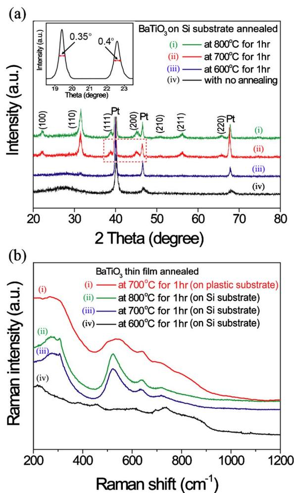
**Figure 2.** (Color online) (a) XRD patterns of BaTiO<sub>3</sub> thin film deposited on Pt/Ti/SiO<sub>2</sub>/Si substrate by rf sputtering and annealed at different temperatures. The inset shows the X-ray rocking curve of BaTiO<sub>3</sub> (111) and (200) peaks. (b) Raman spectra of MIM structures deposited on Si substrate (black, blue, and green lines) and fabricated on plastic substrates (red line).
