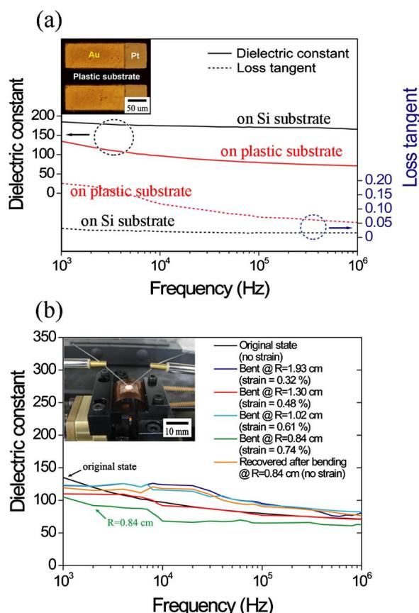
**Figure 3.** (Color online) (a) Dielectric properties of MIM structured BaTiO<sub>3</sub> thin film as a function of frequency on both Si and plastic substrates. The inset shows the optical image of the actual devices fabricated on plastic substrates. (b) Dielectric properties of BaTiO<sub>3</sub> thin film on plastic substrate at different bending radii and their corresponding strains. The inset shows the optical image of mechanical bending stage.
